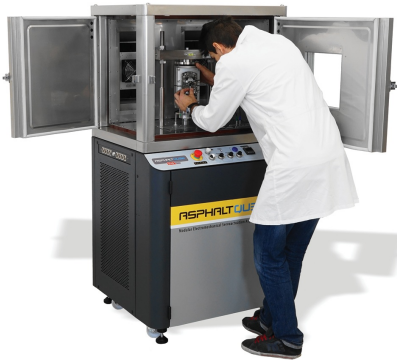
AsphaltQube fitted with Overlay testing jig
